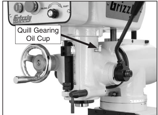
Figure 55. Quill gearing oil cup.
